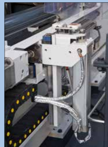
Underside web scribing device
